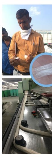
bed out, other smaller impurities are removed and the fibres are combed extremely evenly together. These combed cards are then suitable for particularly fine and shiny yarns such as those usually used for satin fabrics
