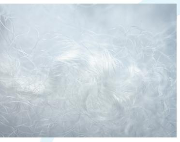
nozzles and processed into fine filaments. The fibres then have a high thermal stability and are heat resistant even at continuous temperatures of up to 200°C. At 230°C, however, a softening process begins to set in. In order to maintain the dimensional stability of the textiles, mangle temperatures should therefore always be below this temperature.
